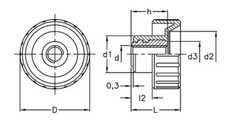
$\begin{array}{ll} d &= 32 \\ d1 &= 17 \\ d2 &= 21 \\ d3 &= 11 \\ d \, 6H = M10 \\ h &= 15 \\ L &= 22.0 \\ l2 &= 9.0 \end{array}$
